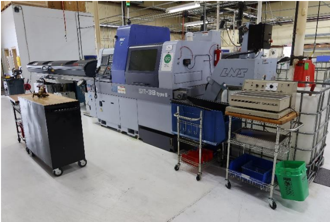
Star SR38 type B (10 Axis Swiss Lathe)
