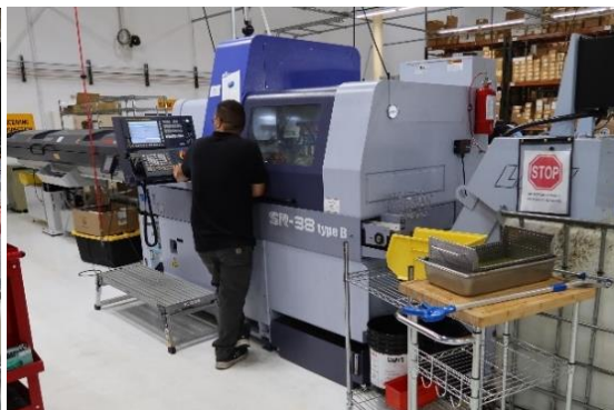
Star SR38 type B (10 Axis Swiss Lathe)
